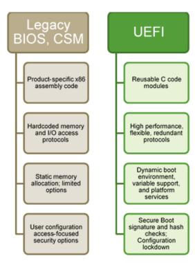
Figure 1: Feature comparison between boot mechanisms
